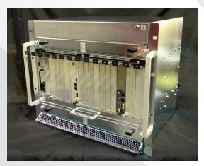
The MicroTCA specification states that an Advanced Mezzanine Card (AMC) module must have a Module Management Controller (MMC). The MMC receives 3.3V management power after the Carrier Manager on the MicroTCA Carrier Hub (MCH) is initialized. The AMC MMCs and system Enhanced Module Management Controllers (EMMCs) can then be powered up and the MCH can communicate with it over the Intelligent Platform Management Interface (IPMI) bus. The Carrier Manager communicates with the MMC on each AMC to
