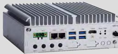
**Product Reference 3, Figure 1.** The UST100-504-FL is a vehicle embedded controller equipped with scalable CPUs including 7th/6th generation Intel® Core™, Pentium® or Celeron® processors for video analytics (Source: **Axiomtek**).
