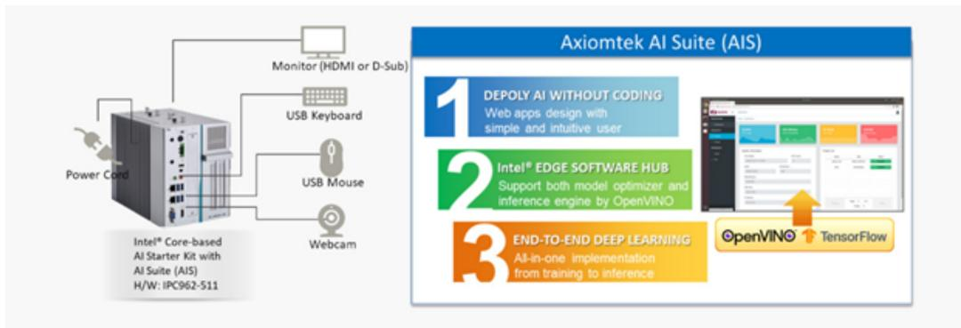
Each Axiomtek/Intel AI Starter Kit comes equipped with a choice of one of our high quality, scalable industrial PCs (IPCs), a camera, and a pre-installed software stack that includes the Intel Training and Learning Suite as well as Intel® Edge Insight for Industrial (EII) Software. The kit is designed to be programmable with web apps. It does not require users to have extensive AI coding experience. It is project development and implementation ready, allowing for fast and successful deployment.
